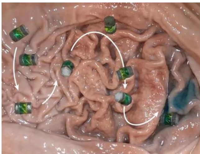
Figure 1 Image showing controlled delivery of liquid medicine by wirelessly controlled origami microrobots in an ex vivo pig stomach. Image credit: Zhao Lab, Stanford U.
